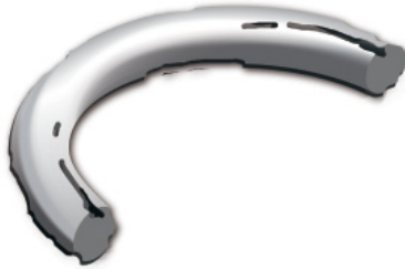
Figure 9-2: Failure due to extrusion and nibbling
