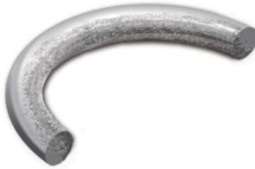
Figure 9-5: Failure due to heat hardening and oxidation
