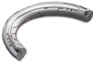
Figure 9-7: Failure due to explosive decomposition
