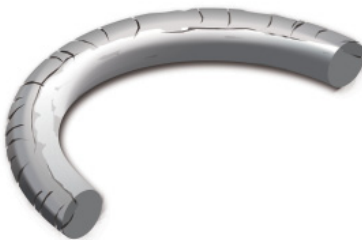
Figure 9-6: Failure due to weathering or ozone cracking
