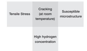
In addition, the weld must cool down to near normal ambient temperature, where the effect of hydrogen is at its maximum. If any one factor is not satisfied, cracking is prevented.
