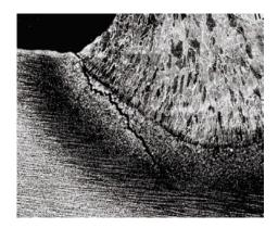
A combination of three factors is necessary to cause HAZ hydrogen cracking:
