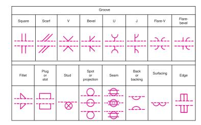
Figure 6-18. Basic weld symbols. (Printed with permission of the American Welding Society)
