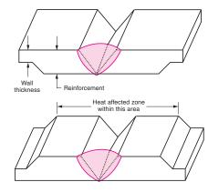
Figure 6-35. The joint thickness and the filler material tensile strength is equivalent to the strength of the base material in this design.
