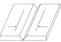
Figure 6-27. Weld joint shrinkage can be determined in four steps. 1. Tack weld the test joint together. 2. Scribe parallel lines, as shown, on approximately 2" centers. Record this dimension. 3. Weld joint with test weld procedure. 4. Measure linear distance and compare with original dimension.
