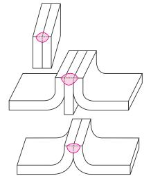
Figure 6-34. Common edge weld joint designs that may be used in fabrication.
