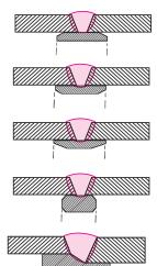
Figure 6-10. Various types of backing rings for pipe joints.
