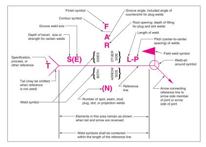
Figure 6-17. The AWS welding symbol conveys specific and complete information to the welder. (Printed with permission of the American Welding Society)
