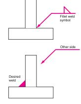
Figure 6-19. Fillet weld symbol shown on the bottom side of the reference line indicates that the weld is located where the arrow points.
