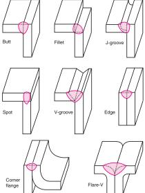
Figure 6-5. Types of welds that may be made with a basic corner joint.
