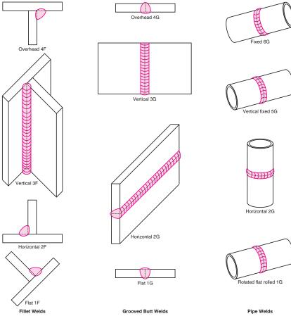
Figure 6-22. American Welding Society definitions of welding positions.
