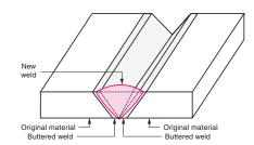
Figure 6-36. Buttering techniques are commonly used to adapt dissimilar metals for welding.
