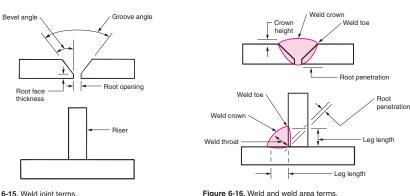
Figure 6-15. Weld joint terms
