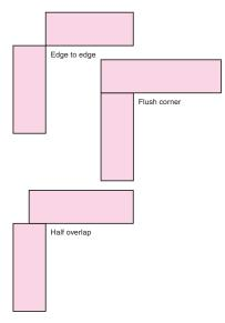
Figure 6-33. Common corner weld joint designs that may be used in fabrication.
